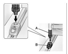
Push both adapter buttons to move the adapters (B) on the straight part of the u-rail. To move the fence around the u-rail, disconnect one side:
